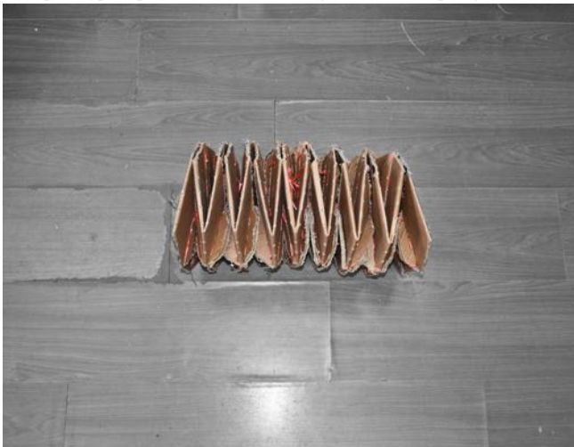
01 A prototype deployable arch with an origami-based morphing mechanism.
