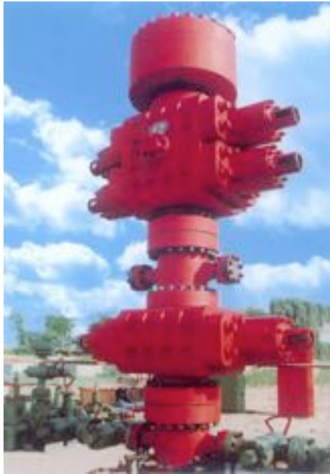
Figure 2: The Deep Sea Horizon (BP) oil spill disaster in the Gulf of Mexico happened when a so-called “blowout preventer valve”, pictured here, failed and large amounts of buoyant crude oil (with dissolved gas) started leaking out and rose towards the surface, entraining some of the surrounding sea water as it rose. Introduction of angular momentum to the entrained seawater might have diminished entrainment and kept the spill within a smallish surface area, easy to collect. Photo source Wikipedia.
