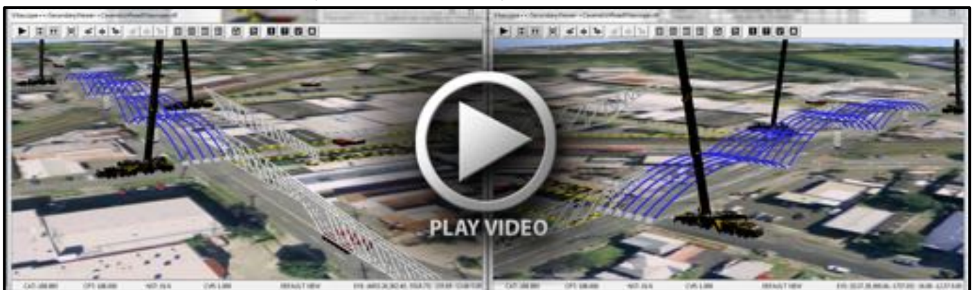
O1a: 3D Animations of Manipulating Trusses of RapidBridgeBuilder (Vitascope++)
